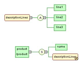
The descriptionLines group is reused in the definition of the product element by clicking the sequence group particle (S) with the Toolbox *Group* tool. The Reference property of the referencing group property sheet is then set to descriptionLines.
