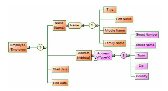
You can edit the properties and child elements of any instance of a complex type defined in the model, and these changes will be propagated to all other instances.
