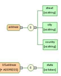
USaddress is a derivation by extension of the address complex type.
